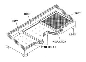
Figure 3: A cabinet solar dryer.
