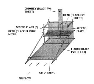
Figure 2: A chimney dryer.
